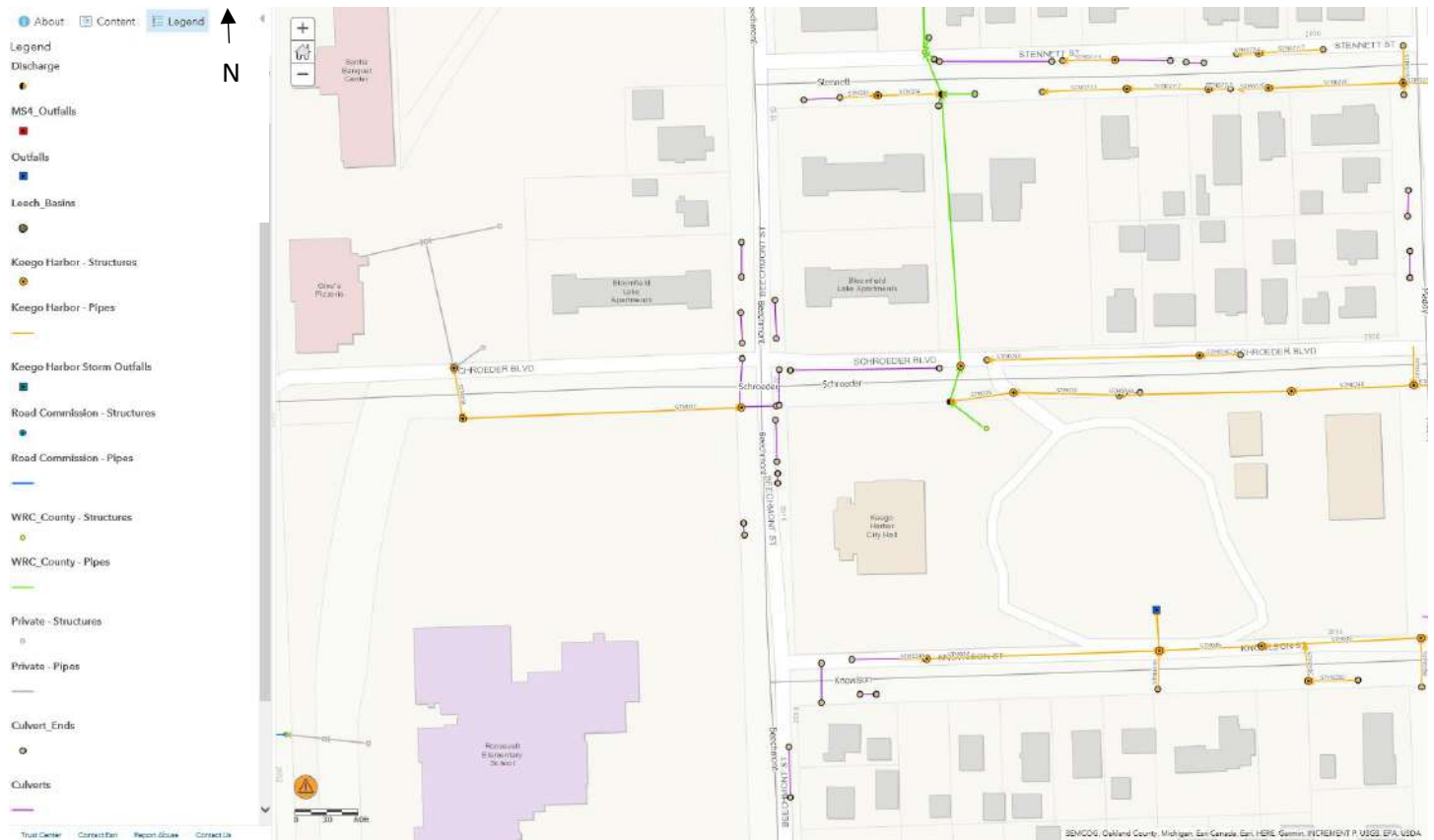
HRC's ArcGIS Map of the existing pipes at the intersection of Schroeder and Beechmont.
